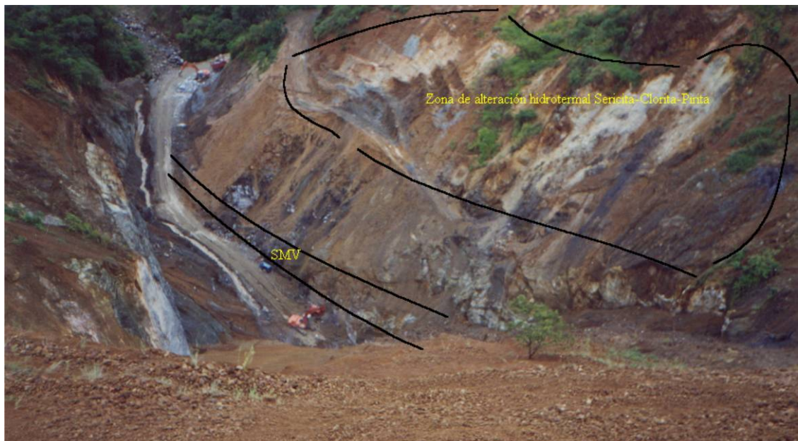
Figure 9.14 Photograph of the La Pastorera pit showing the location of the sericite-chlorite-pyrite alteration zone and the massive sulphide (Source: Alfonso and Cano, 2000)
