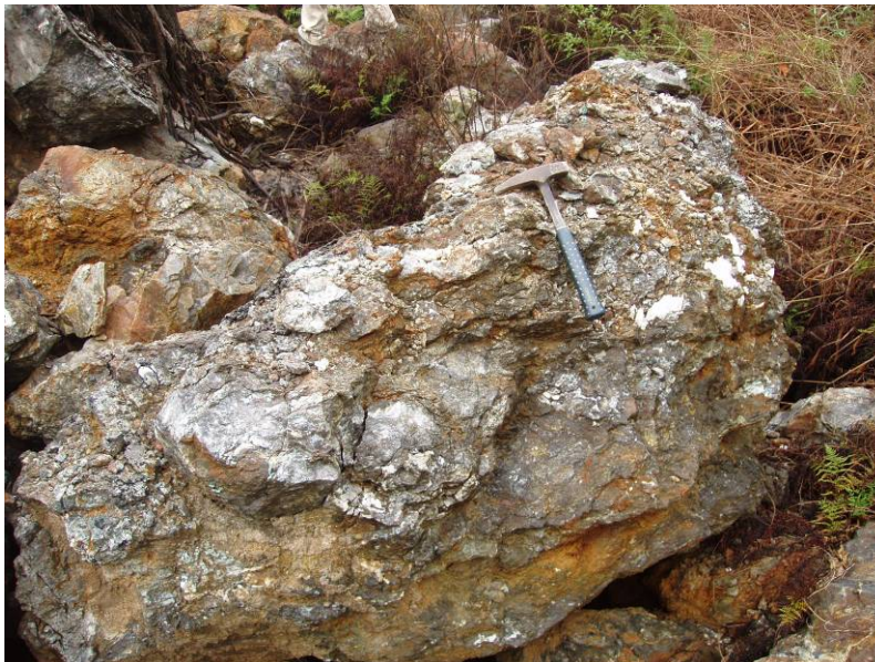
Figure 9.11 Large boulder of massive sulphide on the waste stockpile at the Exman gypsum mine. The sample contains both siliceous and massive sulphide material, sulphide rich zones are weathered to brown iron oxides. Snowden samples 305-1, 305-2 and 305-3 were collected from this boulder (Source: Snowden site visit, 2010)
