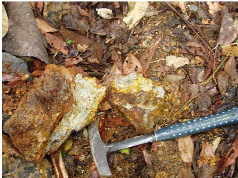
Figure 14.4 Photograph of an oxidised boulder in the Maluca tributary which may represent weathered massive sulphide material. Orange brown areas are weathered iron oxides and may represent oxidised sulphide mineralisation. Snowden sample number 306-1 and 306-2 (Source: Snowden site visit, 2010)
