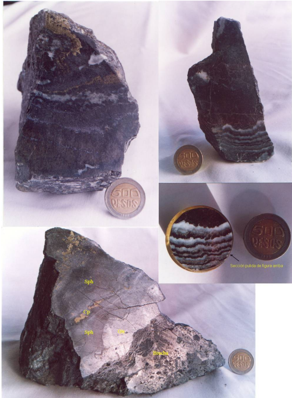
Figure 9.9 Photographs of polished sections of massive sulphide material from La Pastorera (Source: Alfonso and Cano, 2000)
